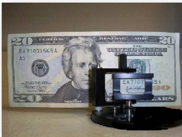
Figure 2 Jasco solid sample holder with $20.00 bill.
