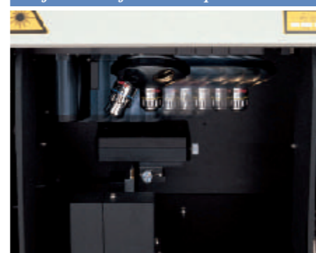
Objective lens for microscopic measurement
